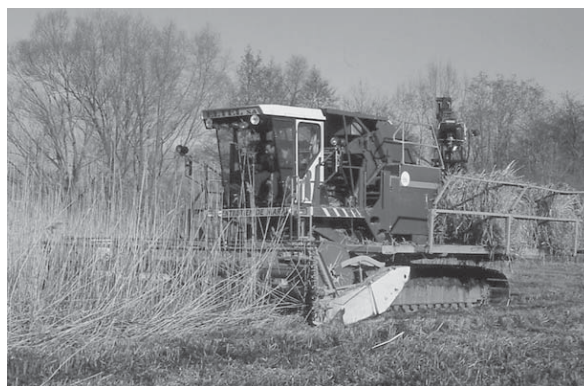
Plate 2. Caterpillar machine used for mowing. The plant material is immediately formed into balls which are loaded on the machine so as to complete the whole management in a single run and thus limit soil damage.
